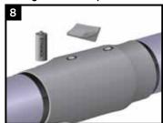
De-grease the surface of the casing using a grease and lint free rag soaked in others.
