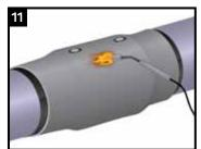
Pre-warm the casing surface around the foaming hole to 40°C. Check the temperature using a temperature measuring device
