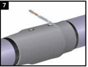
Using a grater, sand down the plugs bringing them flush to the surface of the casing.
