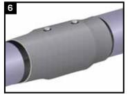
After the foam has hardened, remove the vent plugs and weld the standard weldable plugs.
