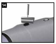
Using a gloved hand or roller, pat down the CFS for about 5 seconds, or until the entire CFS surface makes good contact with the casing.
