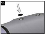
Place the CFS onto the pre-cleaned and pre-warmed section of casing directly over the centre of the foaming hole.
