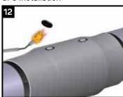
Heat the adhesive side of the CFS with a medium intensity flame until the adhesive turns glossy thus indicating that the adhesive has been activated.
