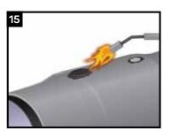
Using a medium flame, heat the backside of the CFS until the adhesive oozes from the edge of the patch.
