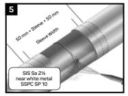
Warm the joint area to 40-50°C before grit blasting. Thoroughly clean the weld area with a grit blaster to "near white metal". Lightly abrade the line coating adjacent to the weld area to a distance 50mm (2") beyond the sleeve width. Wipe clean or air blast the steel and coated areas to remove foreign materials.
