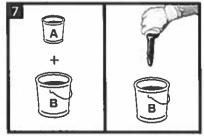
Components must be warmed to at least 20°C (68°F) prior to mixing.
