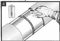
Clean exposed steel and adjacent pipe coating with a non-oily solvent cleanser (ie. ethanol, MEK, etc.) to remove the presence of oil, grease, and other contaminants.
