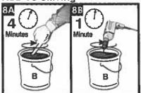
A. Begin mixing slowly. After initial mix has been achieved, a spatula or mixing stick should be used to remove any resin from the side of container.
