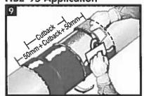
Use a brush, roller or trowel to apply HBE-95 to the joint or patch area to a specified minimum thickness. Cover at least 50mm (2") of the mainline coating. Coating should only be applied at temperatures above 10°C (50°F) and when the amblent temperature is 3°C (5°F) above the dew point. See "Useful Application Information" for other application temperature criteria. Note: Pipe substrate can be pre-heated to 85-95°C (180-200°F) in order to accelerate curing or to cure in cold conditions.
