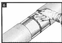
Wipe clean with a lint-free cloth or air blast the steel and pipe coating to remove foreign contaminants. Surface must be clean and dry prior to application of HBE-95.
