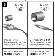
Canusa recommends the use of induction or infrared heating equipment for pipe sizes greater than 760mm (30") 0.D.
