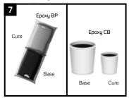
Follow the preparation, mixing and applications instructions provided with the supplied Canusa Liquid Epoxy Pack. For bulk quantities, mix the epoxy cure with epoxy base (see Liquid Epoxy Product data sheet for mixing ratio). Stir for a minimum of 45 seconds to assure uniform
