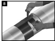
Apply mixed epoxy to a uniform specified thickness of 4-6 mils (100-150 microns) on all exposed bare metal plus 10mm (0.5") onto the adjacent pipe coating using the applicator pads as supplied or an approved tool. Do not apply the epoxy to the mainline coating.
