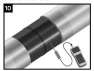
Check the temperature to ensure the preheat has been obtained on the entire pipe circumference. This preheat will substantially cure the epoxy and ensure proper flow and bonding of the sleeve adhesive. Ensure that the epoxy is dry to the touch prior to sleeve installation.
