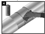
Ensure that the mainline coating edges are beveled to 30° minimum. If there is the presence of oil, grease, or other surface contaminants; clean the exposed steel and adjacent pipe coating with an approved solvent cleanser.
