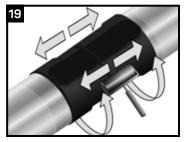
While the sleeve is still hot and soft, use a hand roller to gently roll the sleeve surface and push any trapped air up and out of the sleeve, as shown above. Continue the procedure by also firmly rolling the closure with long horizontal strokes from the weld outwards.
