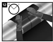
Place the underlap of the sleeve onto the joint, centering the sleeve such that the sleeve overlap is positioned at either the 10 or 2 o'clock position. Press the underlap firmly into place and use a roller to work out any trapped air. Feed the remaining length of sleeve under the nine.
