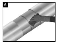
Using a dry, grease and lint-free cloth, wipe clean or air blast the steel and coated areas to remove foreign materials. If necessary, provide additional heat to ensure the surface temperature is 40-50°C (104-120°F).
