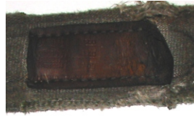
Capacity tag is missing or illegible
