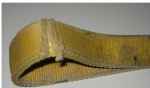
Cuts on the Face of the webbing
