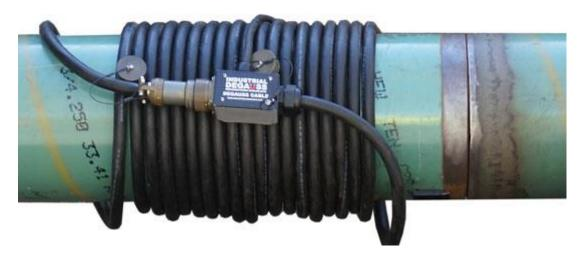
The Degauss Cable has two (2) multipin connectors that mate to form a coil. To mate the multipin connectors, line up the key of the receptacle and the keyway of the male plug and push on the plug. Then align the 3 bayonet rivets on the collar of the male plug to the slots on the receptacle, and twist clockwise to tighten the connection. Only tighten the collar by hand. DO NOT use hand tools or the connectors will be damaged.
