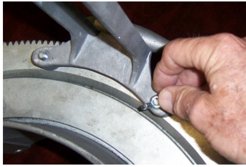
Picture 6 – Installation of the Wing Nut
