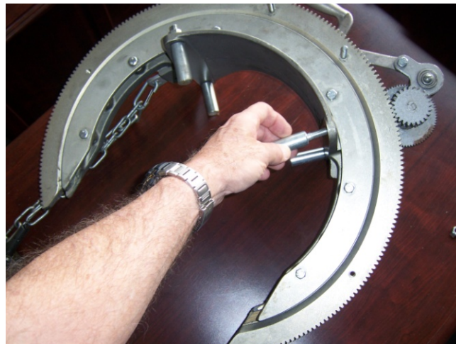
Picture 2 – Spacer Bolt Installation
