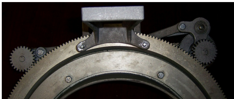
Picture 5 – Installation of Torch Arm on the Threaded Stud
