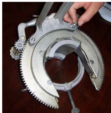
Picture 5 – Installation of the Wing Nut
