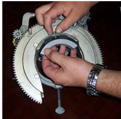
Picture 2 – Installation of Spacer
