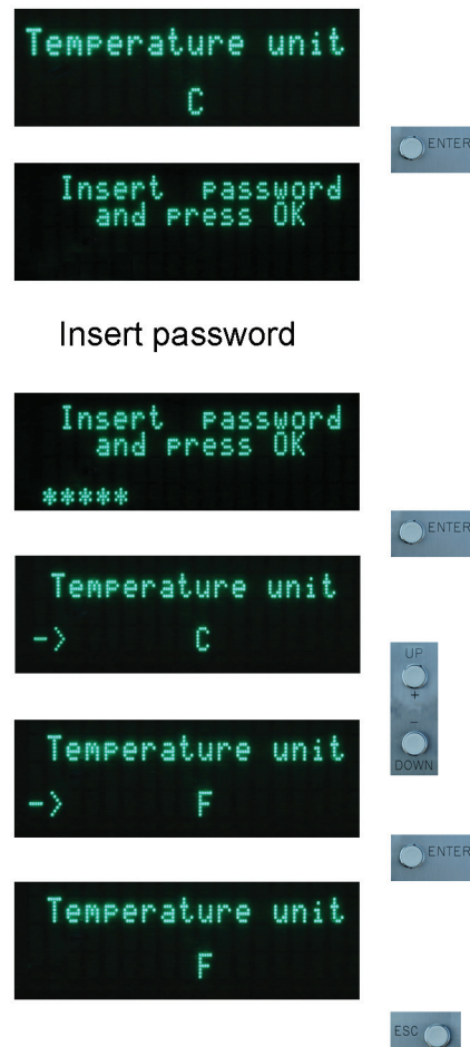
Figure 6.5 - Visualization and setting of the value of a password protected parameter (flow diagram)
