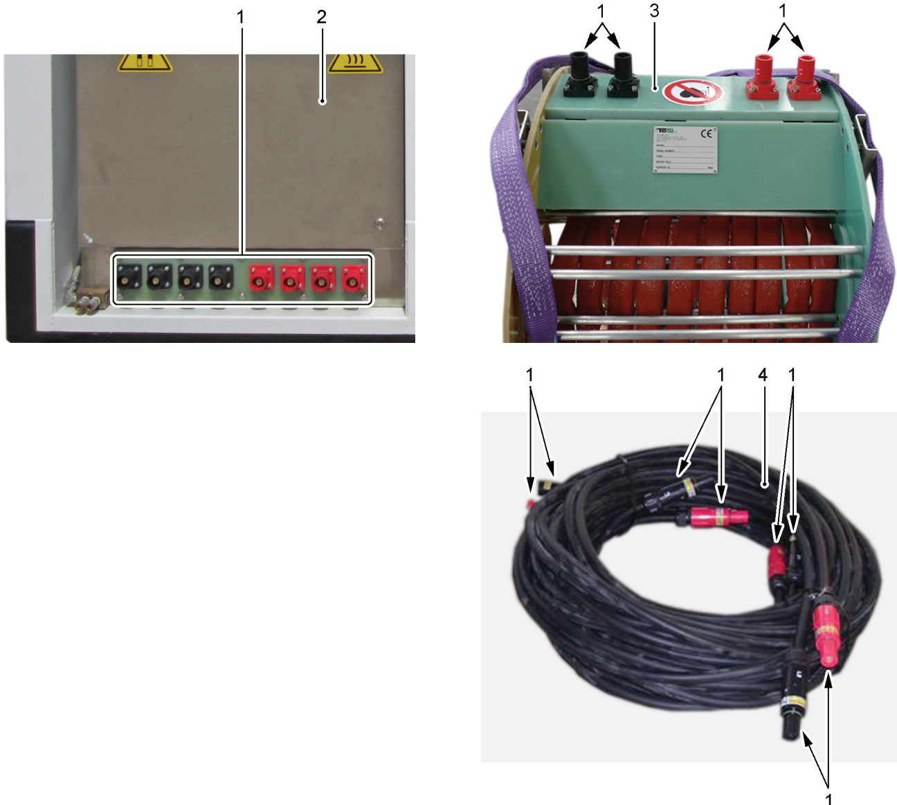
Figure 7.10 - Check the power connectors, situated on the generator, on the coil and on the power cables between generator and coil
