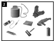
Propane tank, hose, torch & regulator; Appropriate tools for surface abrasion and cleaning (60-80 grit sand paper and a power wire or hand wire brush); Knife, roller, clean white rags & approved cleaner; Digital thermometer with suitable probe; Standard safety equipment; gloves, goggles, hard hat, etc.
