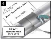
Ensure that the pipe is dry before cleaning. Thoroughly clean the weld area with a sand or grit blaster to "near white metal" SIS Sa  $2\frac{1}{2}$  or equivalent. Using a grinder with a grind disk with rough-ness rating of 40-60, ensure that the PP mainline coating edges are beveled to 15° from the horizontal and that the adjacent PP pipe coating is cleaned, exposing fresh PP, to a distance of 25mm beyond the sleeve width.
