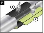
Wrap the sleeve loosely around the pipe, ensuring the appropriate overlap. Ensure that the overlap of the sleeve is a nominal width of 75mm (minimum acceptable width is 50mm). Before finishing wrapping the sleeve: (1) heat the backing side of the underlap until the backing starts to recover (2) heat the adhesive side of the closure until the adhesive appears glossy.
