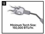
Use moderate flame intensity for sleeve shrinking. Remove protective shields prior to next step. heat
