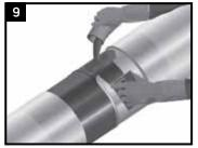
Apply mixed epoxy to a minimum uniform thickness of 6 mils (150 microns) on all exposed bare metal plus FBE toe only, using the applicator pads as supplied or an approved tool.
