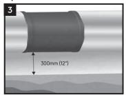
Pipeline must be excavated sufficiently to allow clearance for wrapping and recovering the sleeve. The recommended minimum clearance between bottom of the pipe and ditch should be 300mm (12"). All local regulations should be considered in regards to proper excavation.
