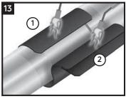
Wrap the sleeve loosely around the pipe, ensuring the appropriate overlap. Remove the remaining release liner from the hold-down strip tape on the underlap of the closure.
