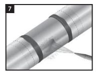
Ensure that the pipe is dry before cleaning. Prepare the steel joint area to a minimum of St3/SP3 (recommended Sa2½/SP10).
