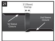
Wrap additional sleeves with a 3" (75mm) overlap and a staggered closure seal position. Recover sleeve starting at overlap of previously applied sleeve with two torches.
