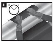
Centre the sleeve over the joint so that the sleeve overlaps between the 10 and 2 o'clock positions.
