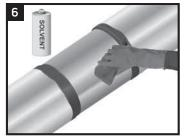
Clean exposed steel and adjacent pipe coating with a solvent cleanser to remove the presence of oil, grease, and other contaminants.
