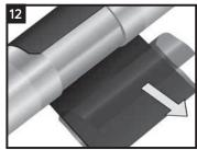
Remove the remaining release liner.
