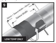
For low temperature installation~0°C (32°F) or when the operating temperature is below 10°C (50°F), use Canusa G Primer 1 US Gal. Stir the Canusa G Primer to ensure the liquid is well mixed before applying. Using a suitable roller or applicator pad, apply the Canusa G Primer to all exposed bare metal and the full width of the sleeve, plus 50mm (2") on each side. Ensure that the primer is applied as a uniform layer.
