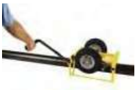
1) Use ratchet to secure Cricket to pipe
